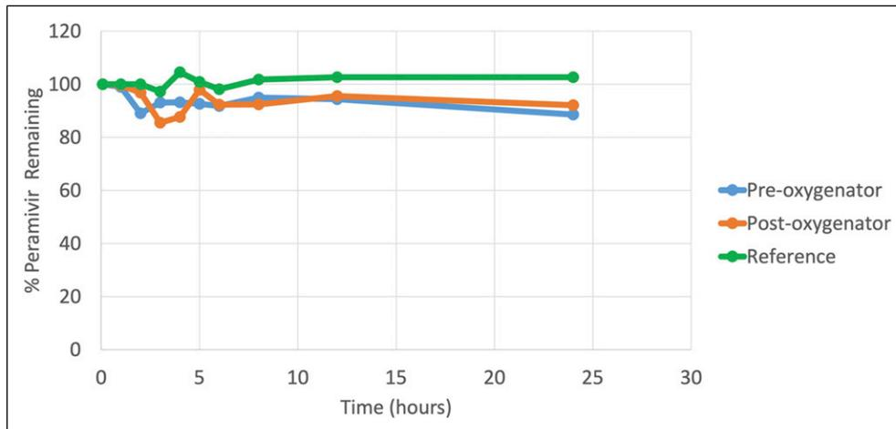
**Figure 1.** Graph of the mean percent of peramivir remaining of pre-oxygenator, post-oxygenator, and reference concentrations versus time in a 1/4-inch extra-corporeal membrane oxygenation circuit with a Quadrox-i pediatric oxygenator.
