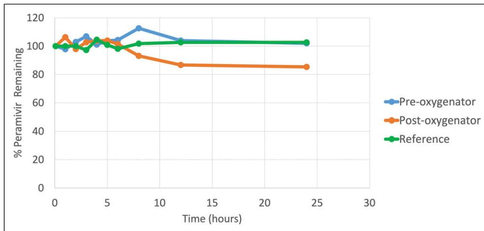
**Figure 3.** Graph of the mean percent of peramivir remaining of pre-oxygenator, post-oxygenator, and reference concentrations versus time in a 3/8-inch extra-corporeal membrane oxygenation circuit with a Quadrox-i pediatric oxygenator.
