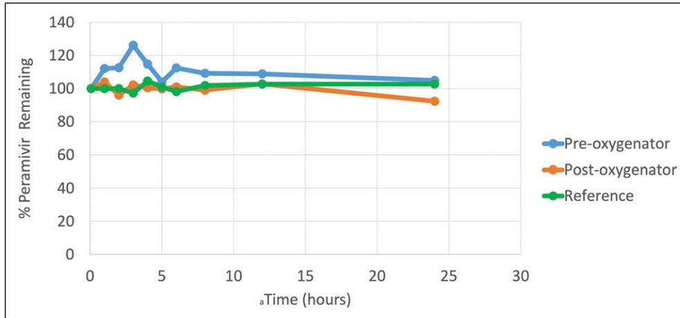
**Figure 2.** Graph of the mean percent of peramivir remaining of pre-oxygenator, post-oxygenator, and reference concentrations versus time in a 1/4-inch extra-corporeal membrane oxygenation circuit without a Quadrox-i pediatric oxygenator.
